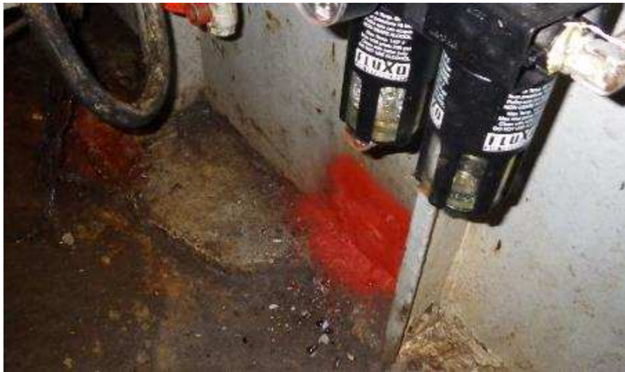
Figure 7- Welded hole from winch room to engine room
