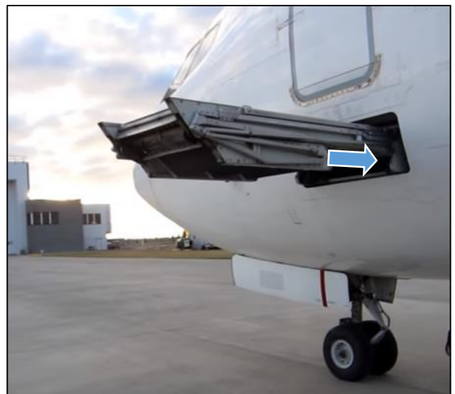
Figure 4: Sequence of airstair retraction (operated via exterior control on these pictures)
