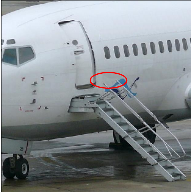
Figure 2: Door in ‘cocked’ position and retracted handrails (red encircled)
