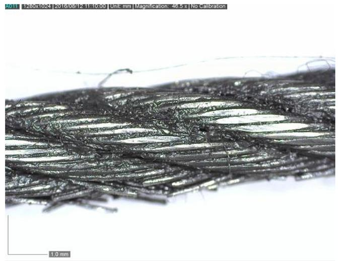
Figure 6: right rudder cable (with grease)
