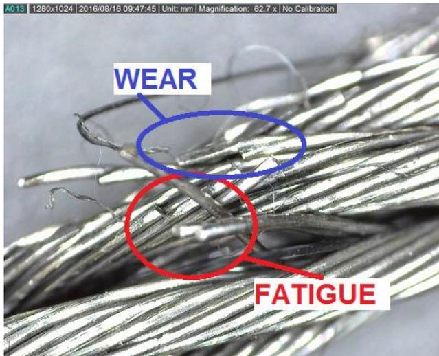
Figure 4: Individual wire strand failure
