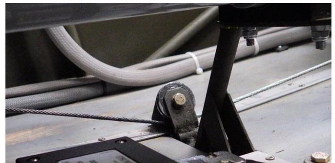
Figure 3: right rudder control cable
