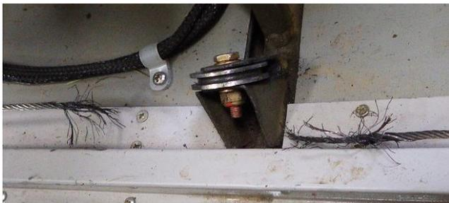
Figure 1: failed left rudder control cable
