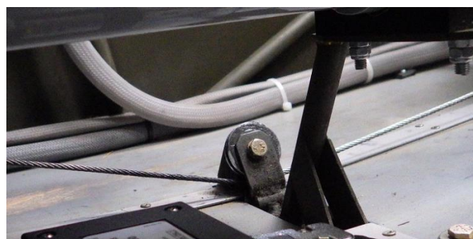
Figure 3: right rudder control cable
