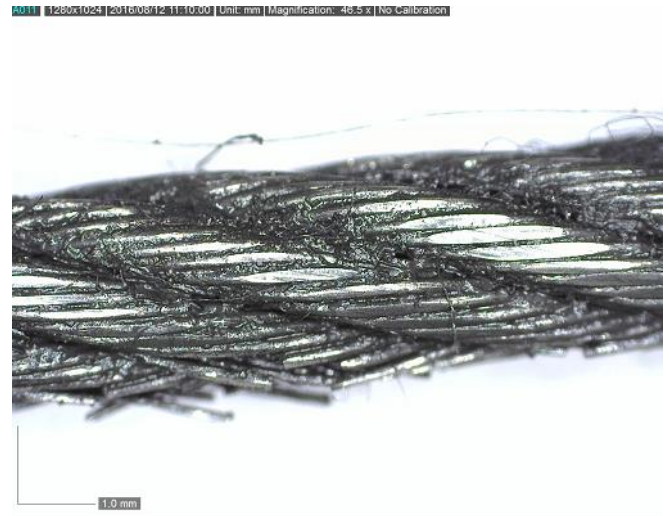
Figure 6: right rudder cable (with grease)
