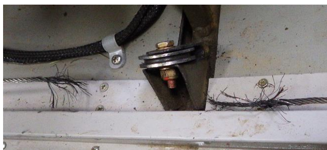
Figure 1: failed left rudder control cable
