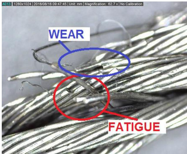
Figure 4: Individual wire strand failure
