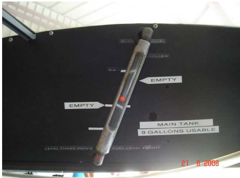
LH Fuel Tank (Main) gage as per STC SA36 RM
