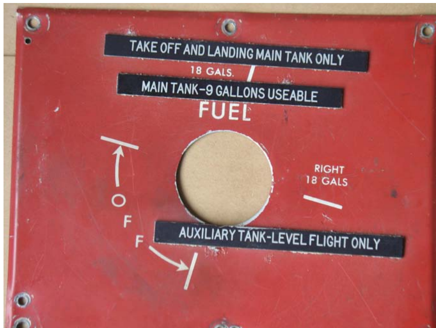
Fuel Tank Selector Valve (Correct configuration as per FAA STC SA 36 RM)
