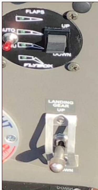
Figure 1: showing the position of the 2 switches (flaps switch above, landing gear switch below) on the center console
