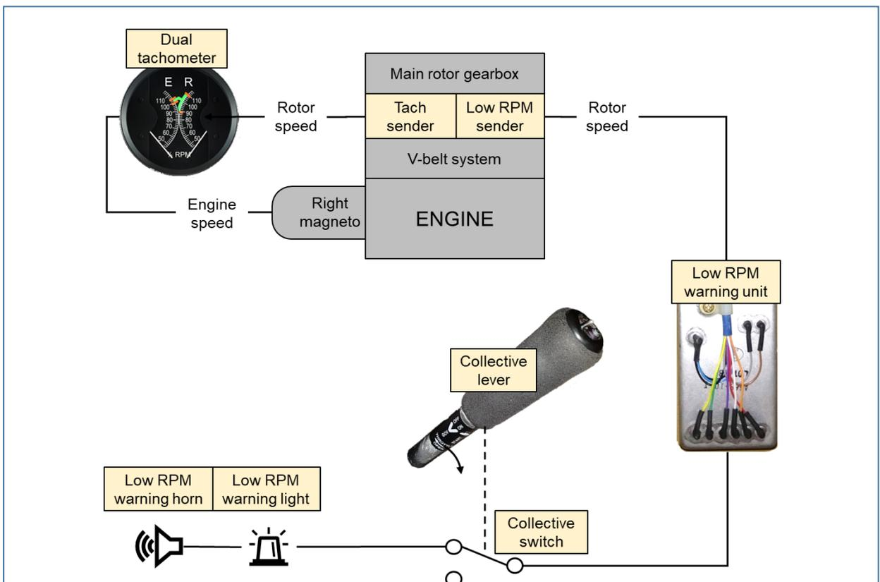
Figure 6 Schematic presentation of the Low RPM warning system
