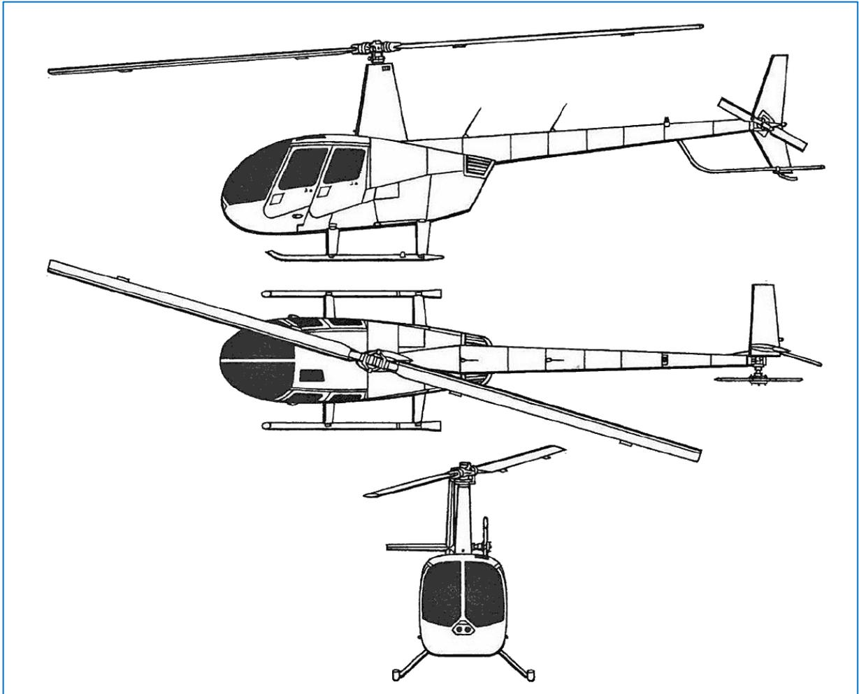
Figure 4 Three-view drawing of the R44
