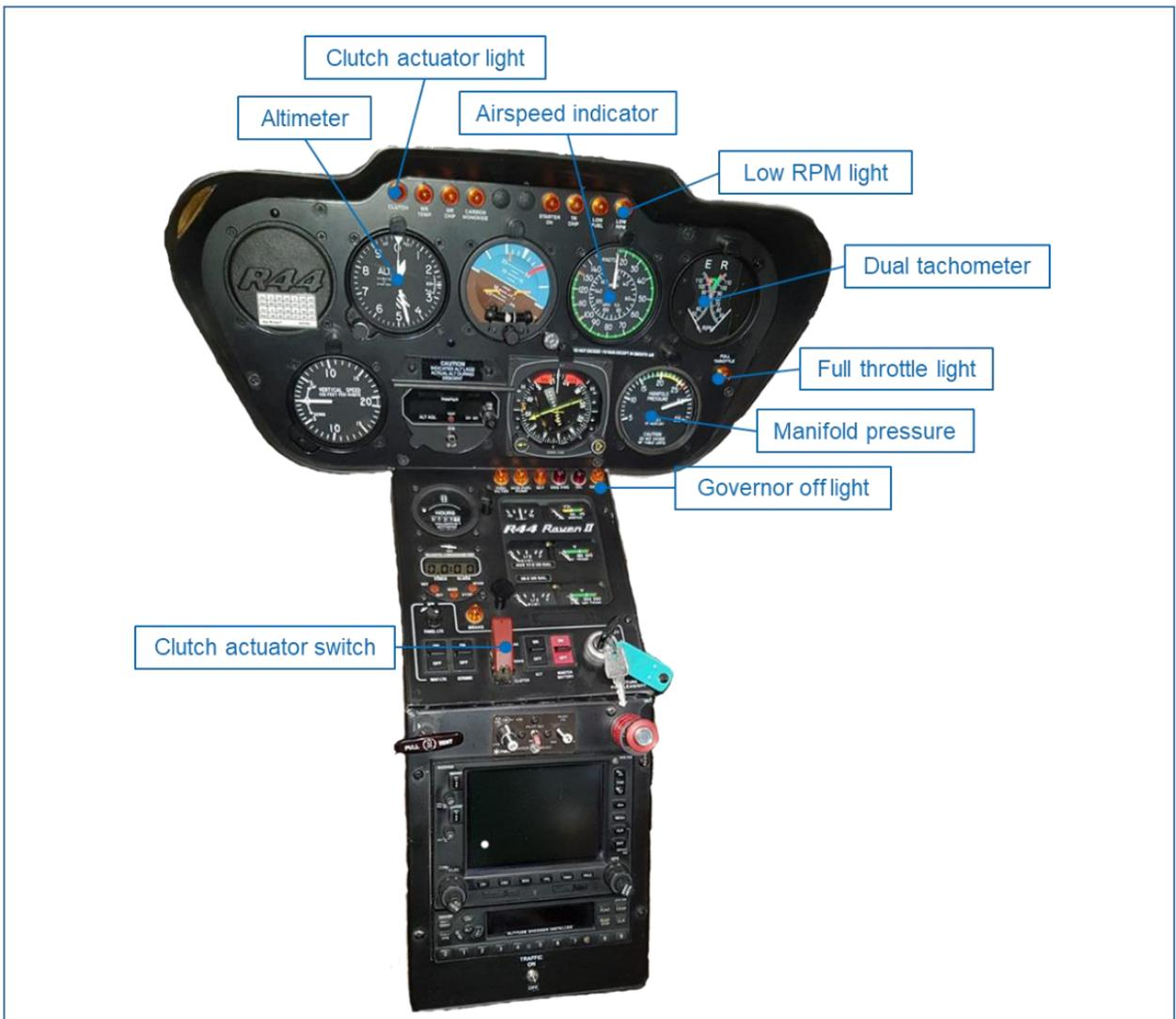
Figure 7 Cockpit panel of the accident helicopter with the relevant warning lights and instruments
