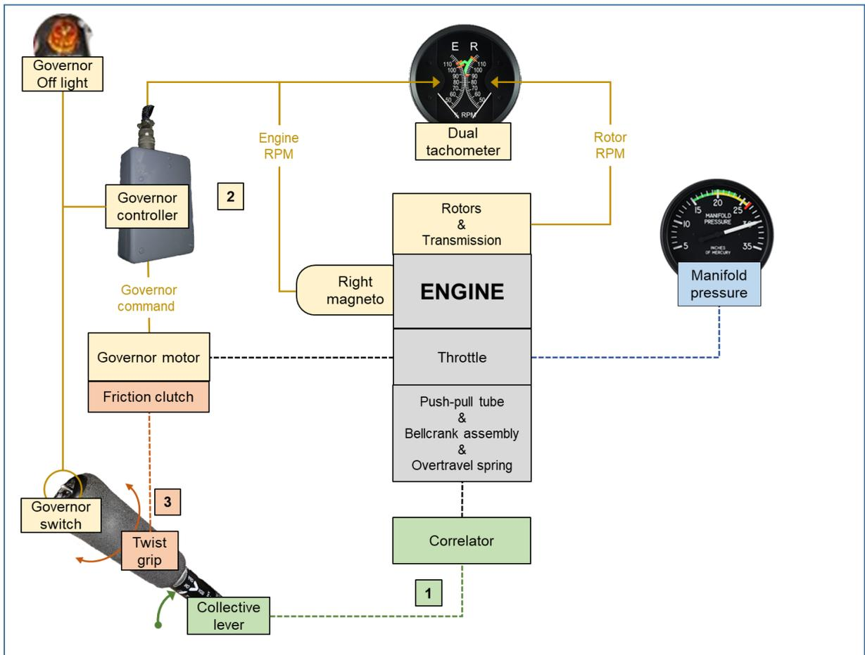
Figure 5 Schematic presentation of the engine throttle control
