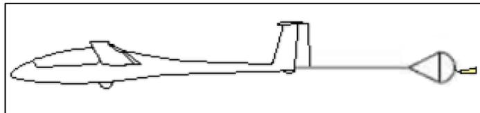
Figure 4: Sketch of a released fin-parachute assembly
