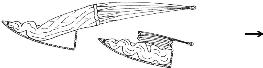
Figure 7: Sketch from the flight manual on how to fold up the parachute in the cover box
