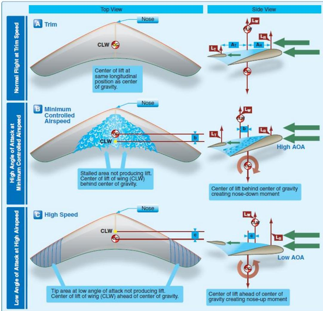
**Figure 25: Trim, minimum controlled airspeed, and high speed pitching moments.**
