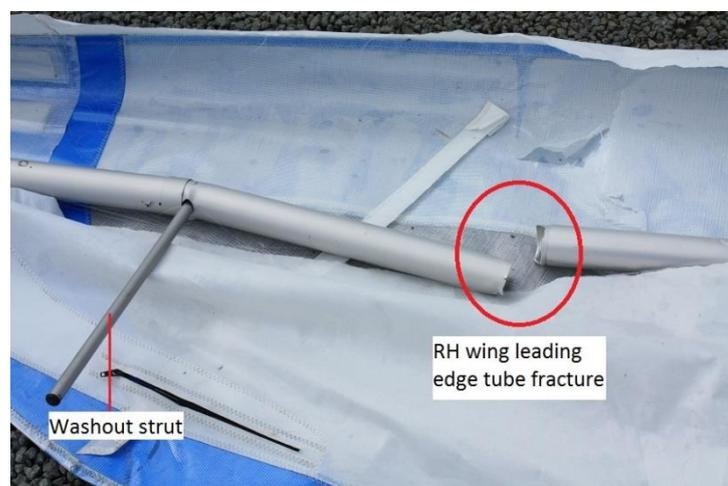
Figure 11: Fracture N°1
