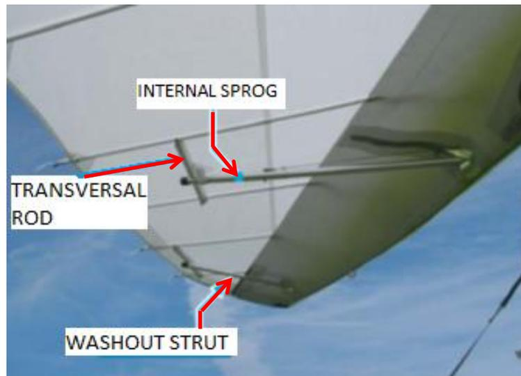
**Figure 3: Typical Reflex System of a wing without king post**
