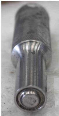
**Figure 6: Peening tool**
