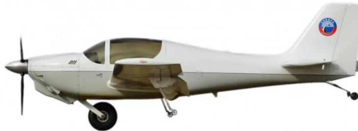
Figure 2 : Europa Classic Monowheel with the flaps and outriggers retracted
