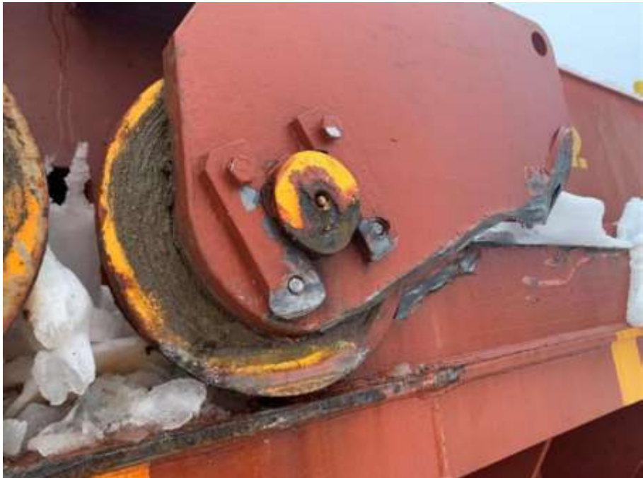
Figure 16 - Damage to the hatch cover of cargo hold N°2
