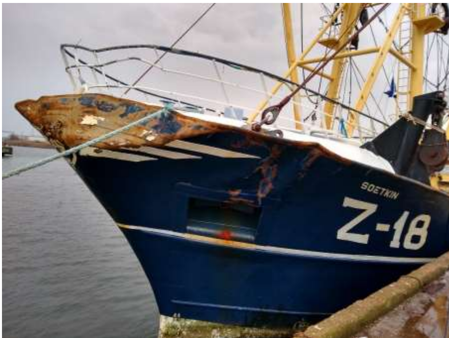
Figure 12 - Damaged bow of the fv Z.18 - SOETKIN
