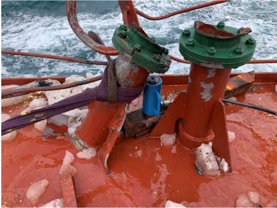
Figure 15 - Damaged air vents of BWT N°1
