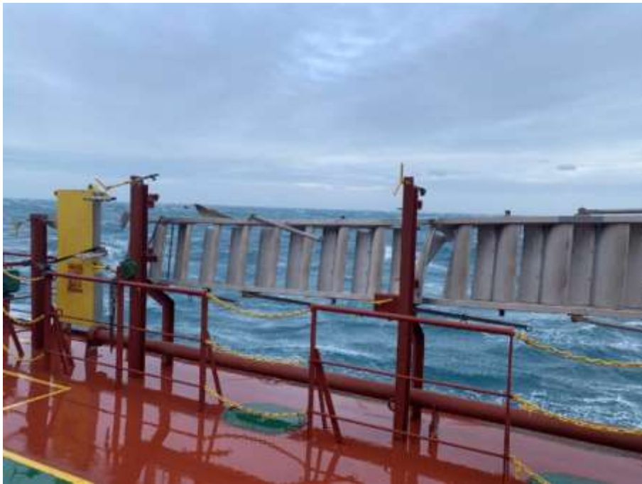
Figure 17 - Damaged accommodation ladder on board mv CALYPSO.GR
