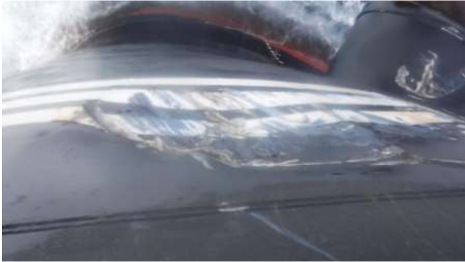
Figure 11 - Indent on SB bow of mv CALYPSO.GR
