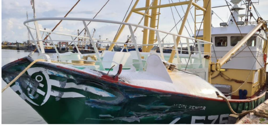
Figure 7 - Fv Z.575-HEIN SENIOR damaged after collision
