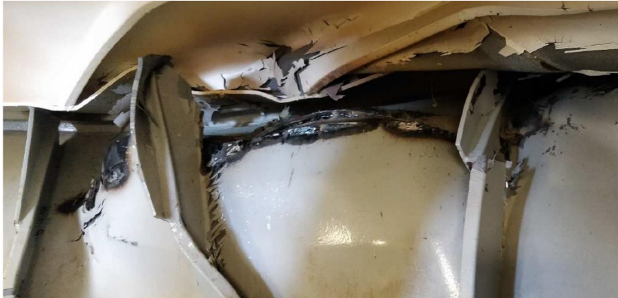
Figure 13 - Upper rupture of the hull of fv Z.575-HEIN SENIOR
