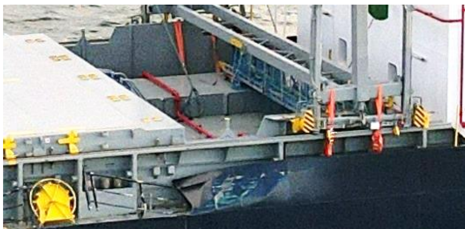
Figure 18 - Damaged railing, bulwark and gantry crane on board mv ACEROMAR
