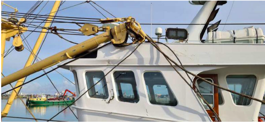
Figure 15 - PS derrick hit the wheelhouse of fv Z.575-HEIN SENIOR
