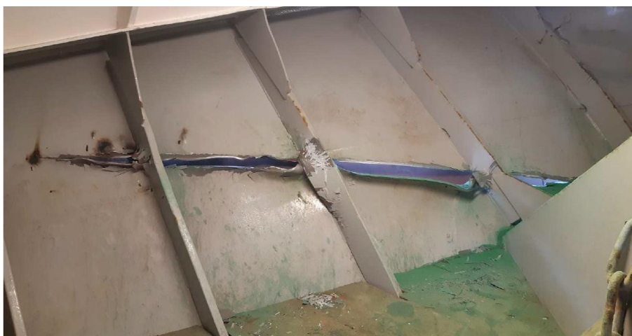
Figure 12 – Lower rupture in the hull of fv Z.575-HEIN SENIOR
