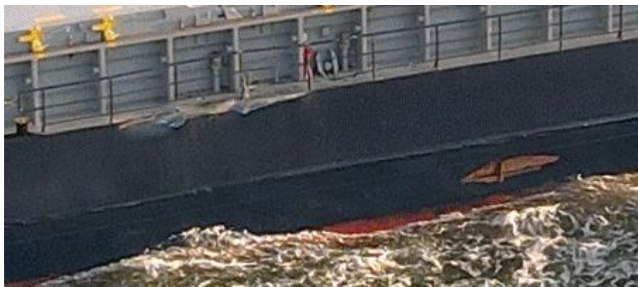
Figure 17 - Detail of damage on PS side plate of mv ACEROMAR
