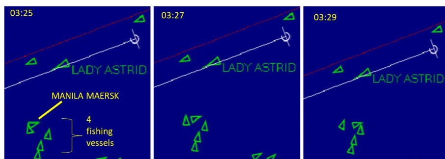
Figure 5 - Radar observation of four fishing vessels crossing the heading of the mv MANILA MAERSK
