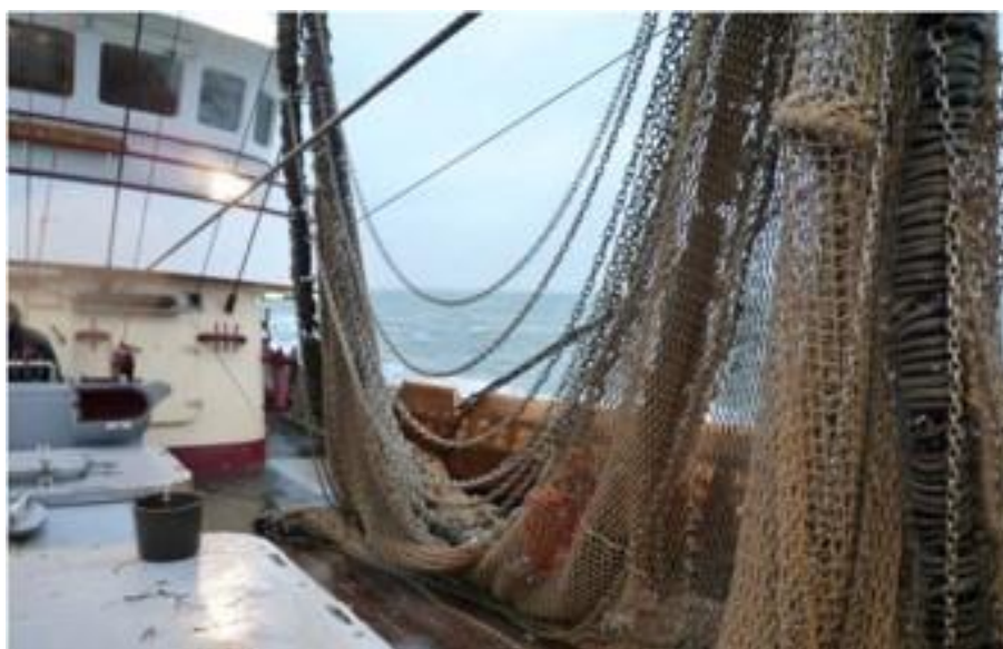
Figure 3 – Example of tickler chains put on deck for inspection
