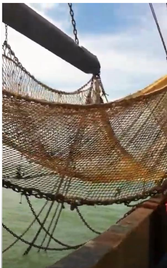
Figure 1 – Sumwing with tickler chains of Z.18-SOETKIN
