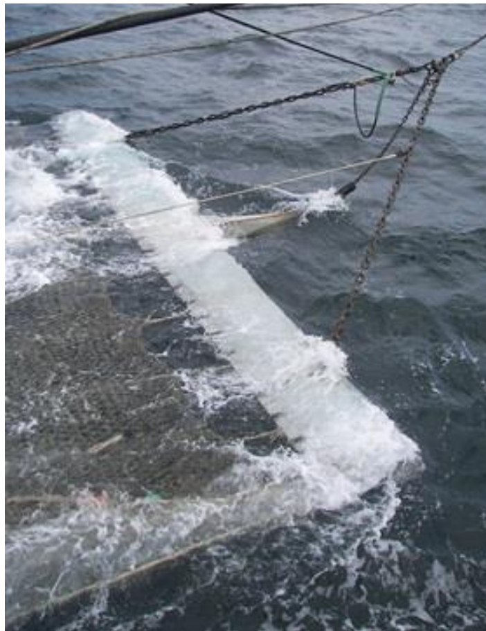
Figure 10 – Sumwing pulled through the water
