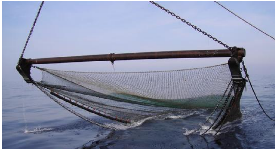
Figure 5 - Trawl beam with skid shoes at the ends
