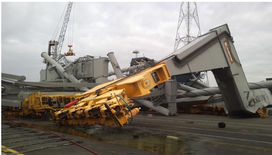
Figure 17 – Collapsed gantry crane
