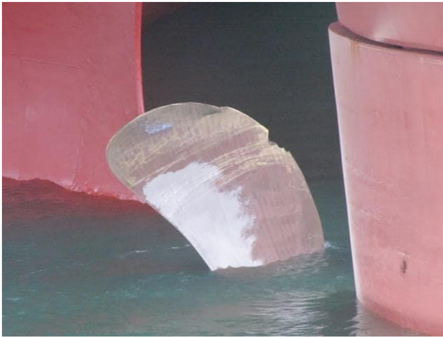
Figure 16 - Damaged propeller of the mv APL MEXICO CITY
