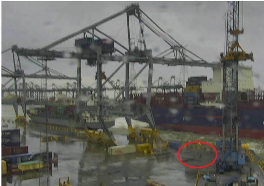
Figure 5 - Gantry crane collapsing and people running for their lives
