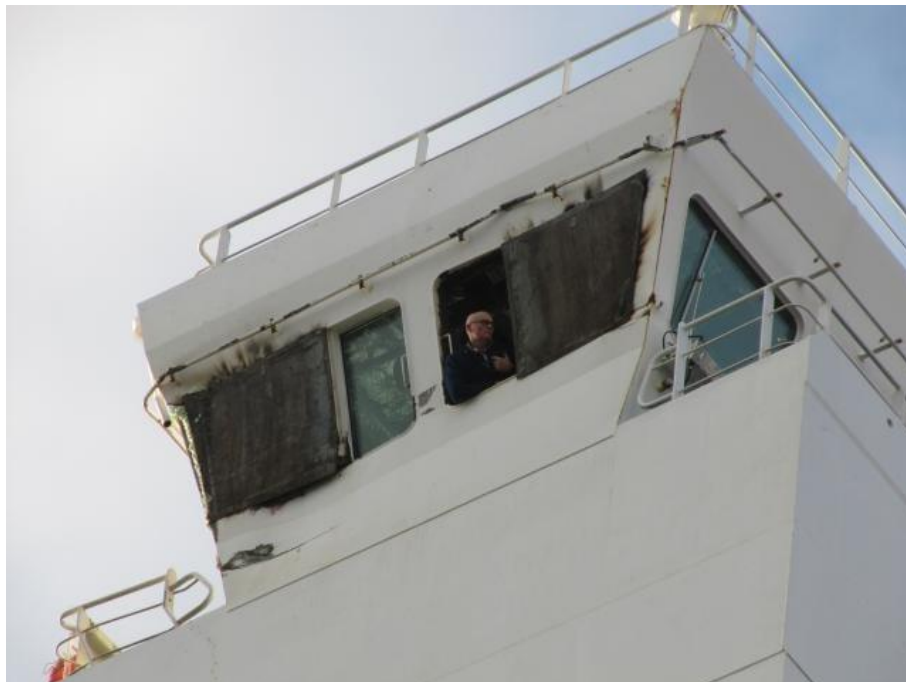
Figure 13 - Damage to wheelhouse of the mv APL MEXICO CITY temporarily repaired
