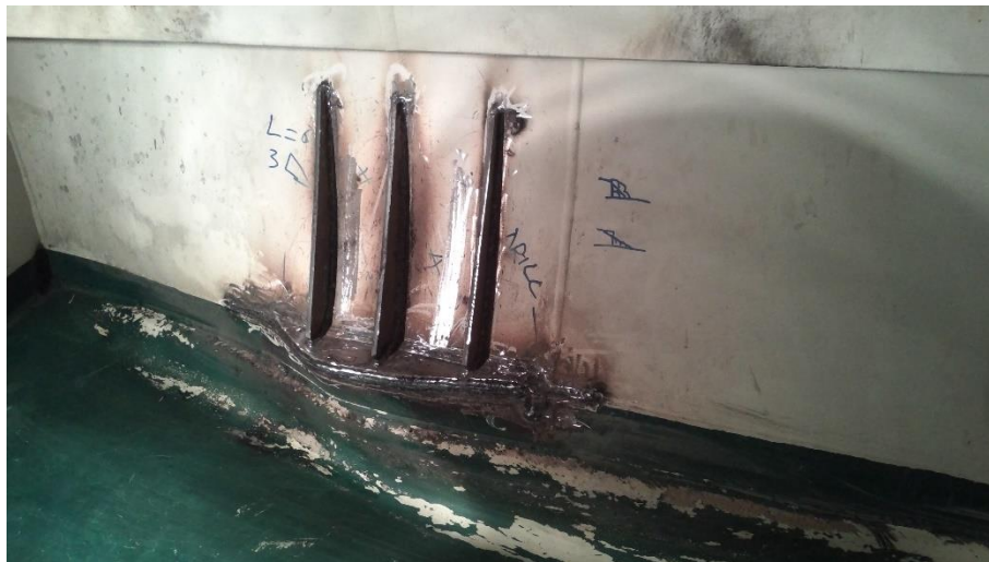
Figure 15 - Temporarily repaired hull of the mv APL MEXICO CITY seen from inside the engine room
