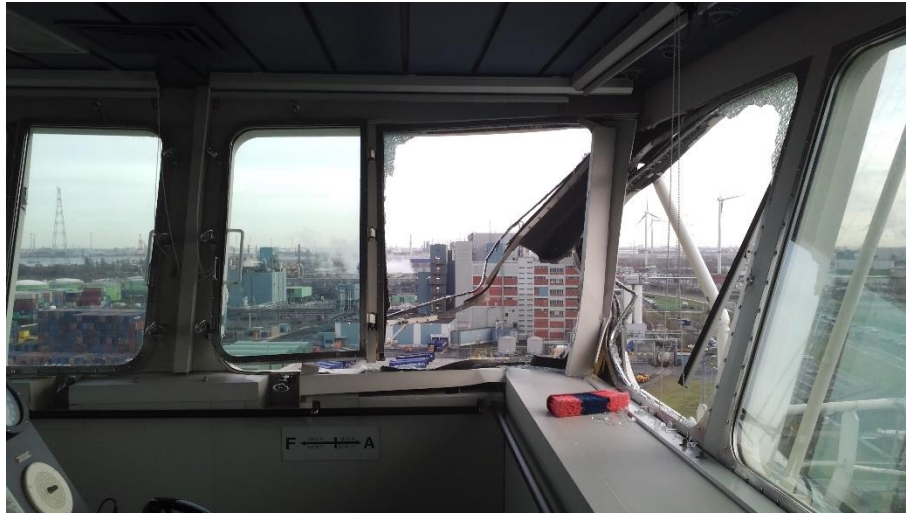
Figure 12 - Damage to the wheelhouse of the mv APL MEXICO CITY seen from inside
