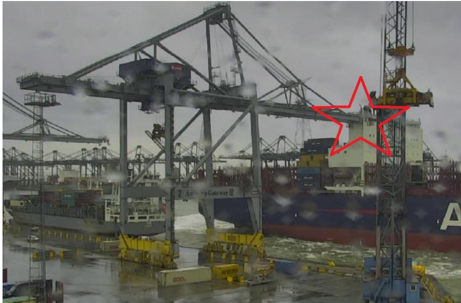
Figure 4 – mv APL MEXICO CITY striking gantry crane
