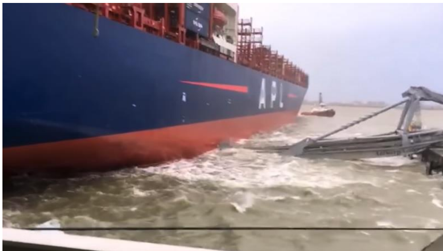
Figure 6 - Jib of gantry crane penetrating hull of mv APL MEXICO CITY during fall
