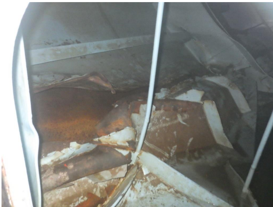
Figure 10- Temporarily repaired damage inside FW tank
