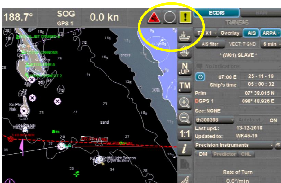
Figure 6 - ECDIS screen, alarms muted
