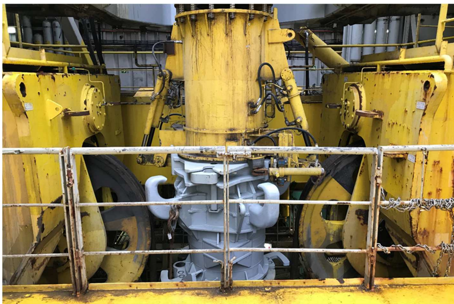
Figure 9 - Gripper holding telescopic pipe
