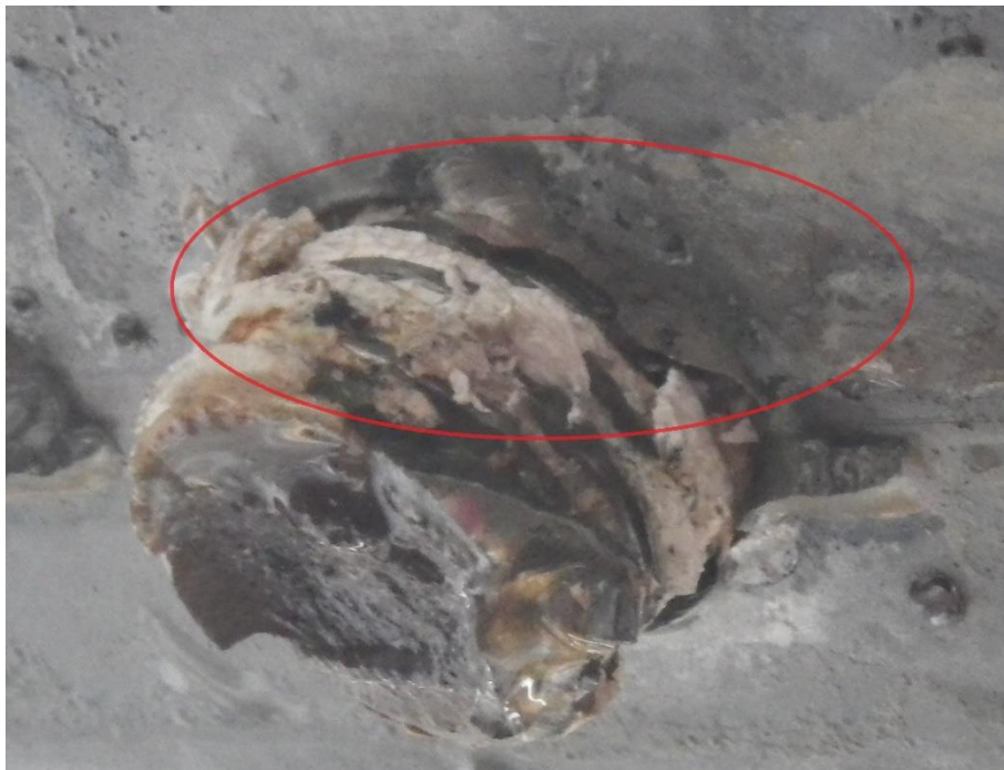
Figure 9 - Part of threaded rod welded to keel plate
