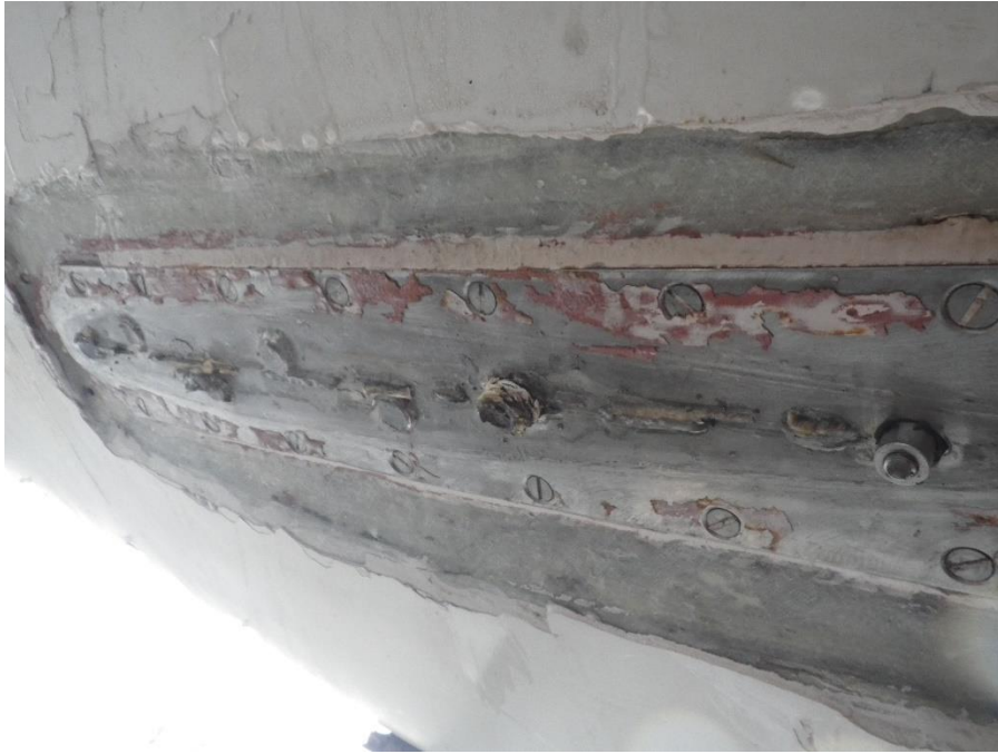
Figure 15 - Keel plate still present on hull with larger part of keel missing
