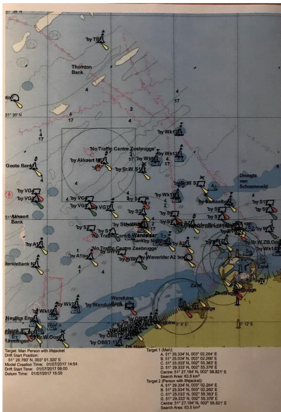
Figure 2 –Search Box Prediction Software screenshot with simulated search box for person with life jacket
