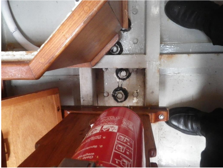
Figure 8 - Nuts and threaded rods and bolts that hold the keel in place seen from inside the sy CAPELLA
