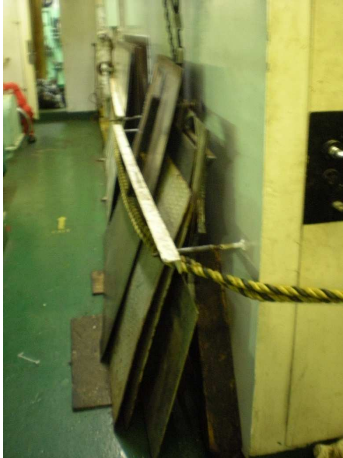
Figure 1 - Normal stowage position of steel plates in engine room
