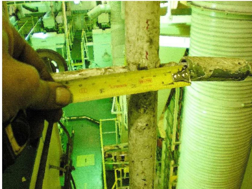
Figure 10 - Male/female connection of railing and maximum insert
