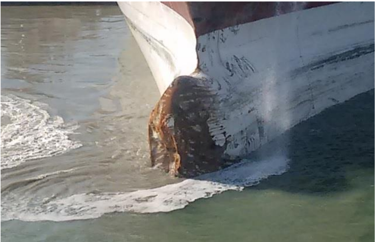
Figure 9 - Damaged bulbous bow of the mts AL ORAIQ after the collision
