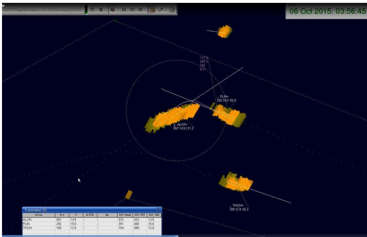
Figure 5 – Imminent collision between mts AL ORAIQ and mv FLINTERSTAR as seen on VTS Radar Images
