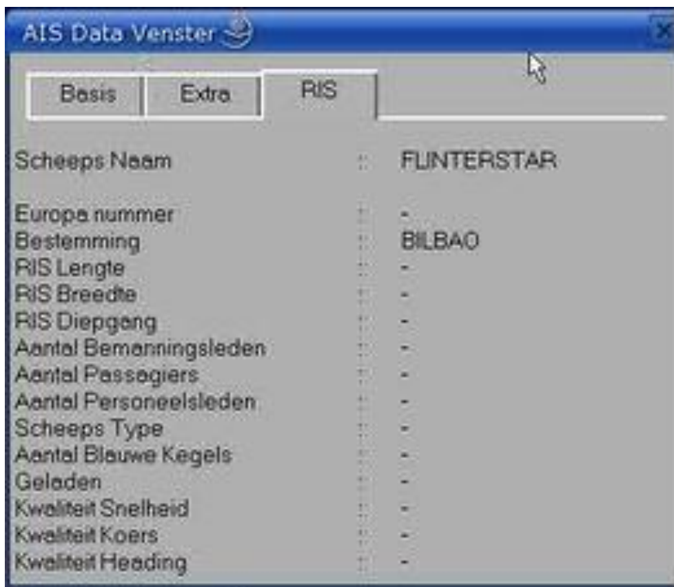
Figure 7 - Detailed Automatic Identification System data from mv FLINTERSTAR not filled out as seen on VTS radar screen
