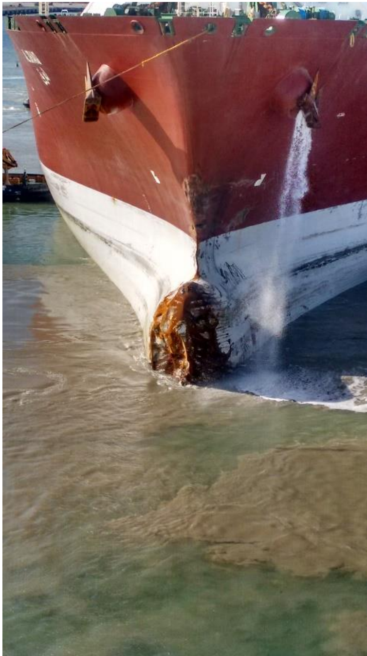
Figure 4 - Damage to the mts AL ORAIQ after the collision
