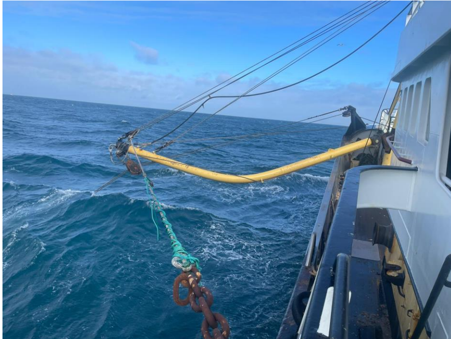
Figure 4 - Damage to PS derrick
